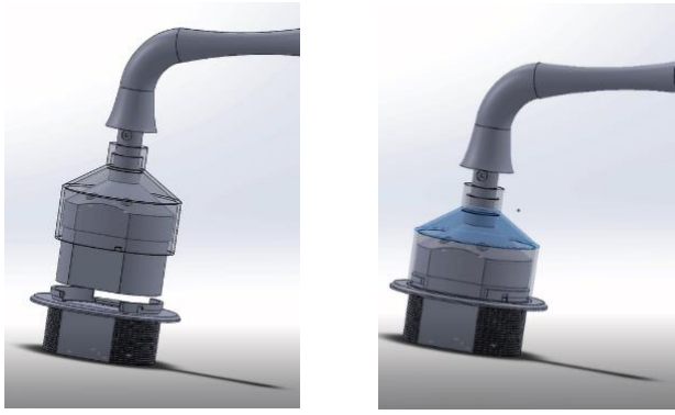
(a) (b) Fig.11 The all-insulated inductive charger
